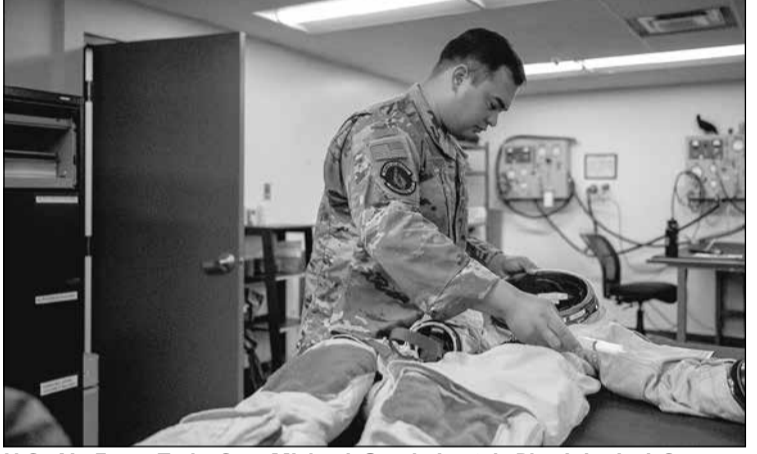
U.S. Air Force Tech. Sgt. Michael Goodwin, 9th Physiological Support Squadron (PSPTS) aircrew flight equipment technician, checks the integrity of one of the full pressure suits used by U-2 Dragon Lady pilots at Beale Air Force Base, California, July 29. Technicians like Goodwin take time to ensure the functionality of the suits are maintained and will test functionality of components to ensure pilot safety. Photo courtesy of U.S. Air Force photo by Charles Borsos
