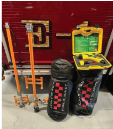
Millis Fire Department's newly obtained EV fire supplies (2 EV fire extinguishing blankets, an EV extinguishing nozzle, and the EV plug). Source: Millis Fire Chief Richard Barrett
