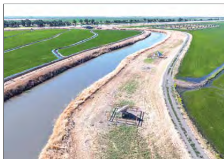
A drone view of newly installed equipment from the California Department of Water Resources’ Sustainable Groundwater Management Office to enhance the monitoring and understanding of land subsidence in California. The newly installed GPS station and remote sensing calibration equipment are firmly anchored into the ground to ensure precise positioning and detect vertical movement of the Earth’s surface. Photo by Nick Shockey / California Department of Water Resources
