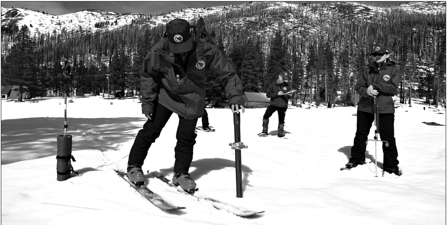
The Department of Water Resources (DWR) recently conducted the third snow survey of the season at Phillips Station. The manual survey recorded 28 inches of snow depth and a snow water equivalent of 11 inches, which is 47 percent of average for this location. Photo courtesy of Department of Water Resources
