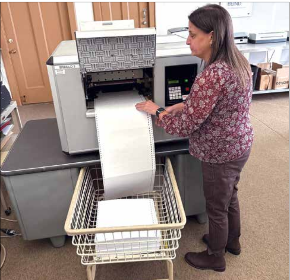
Jill Guilbeau, manager of Society for the Blind's braille production program, creates a brailled document using the Braillo2 machine in the Sacramento office. Photo courtesy of Society for the Blind
