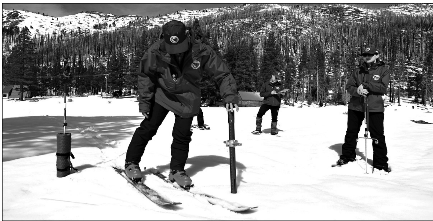
The Department of Water Resources (DWR) recently conducted the third snow survey of the season at Phillips Station. The manual survey recorded 28 inches of snow depth and a snow water equivalent of 11 inches, which is 47 percent of average for this location. Photo courtesy of Department of Water Resources
