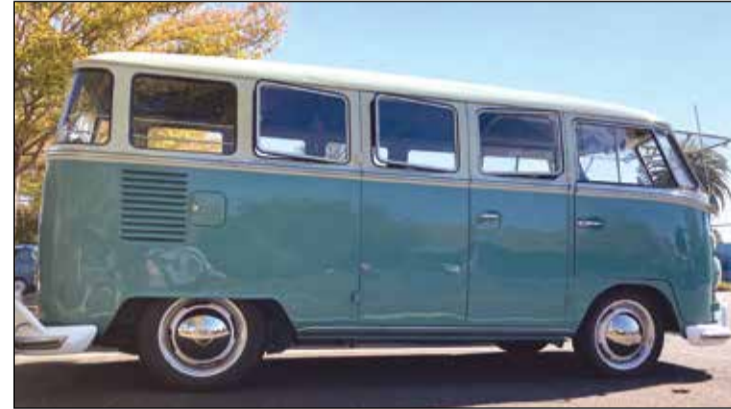
This 13-window Deluxe model has flip-up "safari" windows in front and extra corner windows in the rear.
