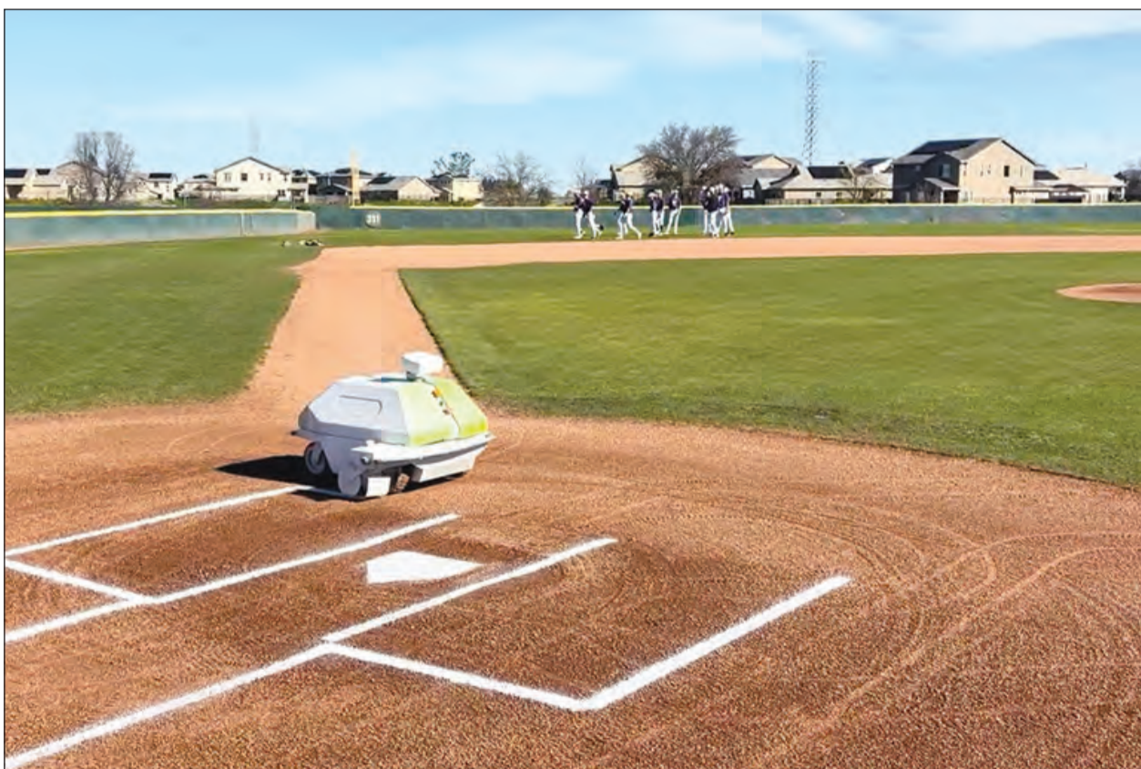
The Turf Tank robot at Bradshaw Christian High School is shown painting field markings on the baseball field. Courtesy photos
