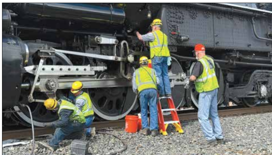
Maintenance workers grease the wheels of Big Boy during its Oroville stop on April 9, keeping the world's largest operating steam locomotive ready for the rails. Photo by Susan Meeker
