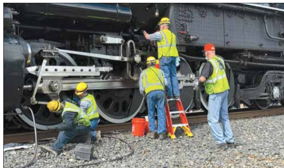
Maintenance workers grease the wheels of Big Boy during its Oroville stop on April 9, keeping the world's largest operating steam locomotive ready for the rails. Photo by Susan Meeker
