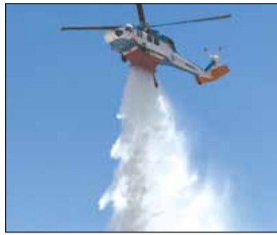
The helicopter is equipped with a 1,000-gallon water tank. Photo courtesy of PG&E
