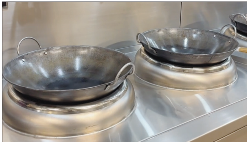
Part of the Sacramento Asian Sports Foundation's new induction kitchen is shown, featuring a four-wok induction station, griddle, two combi ovens, deep fryer and stock pot station. Photos courtesy of SMUD
