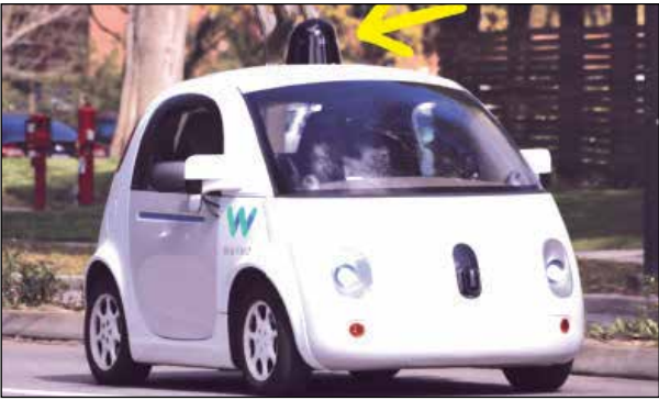
This is a prototype self-driving car. It cruised around Mountain View, California in 2017. The black, gumball-shaped device on top contains some of the car’s sensors. There are sensors all over the car, too. Grendelkhan CC BY-SA 4.0, arrow by Dr. Universe
