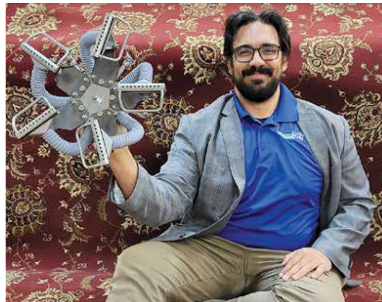
Colonial ChemDry's new owner Michael Halliday with the powerhead star tool that sprays a cleaning agent and agitates it to extract dirt from carpets.
