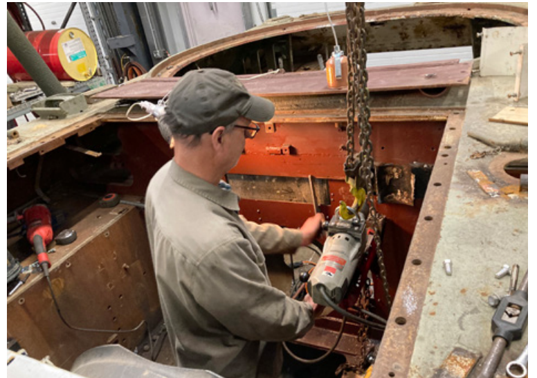
Volunteer Jim Winroth works with the newly rebuilt cabin firewall in the M36 Jackson Tank Destroyer at the American Heritage Museum.
